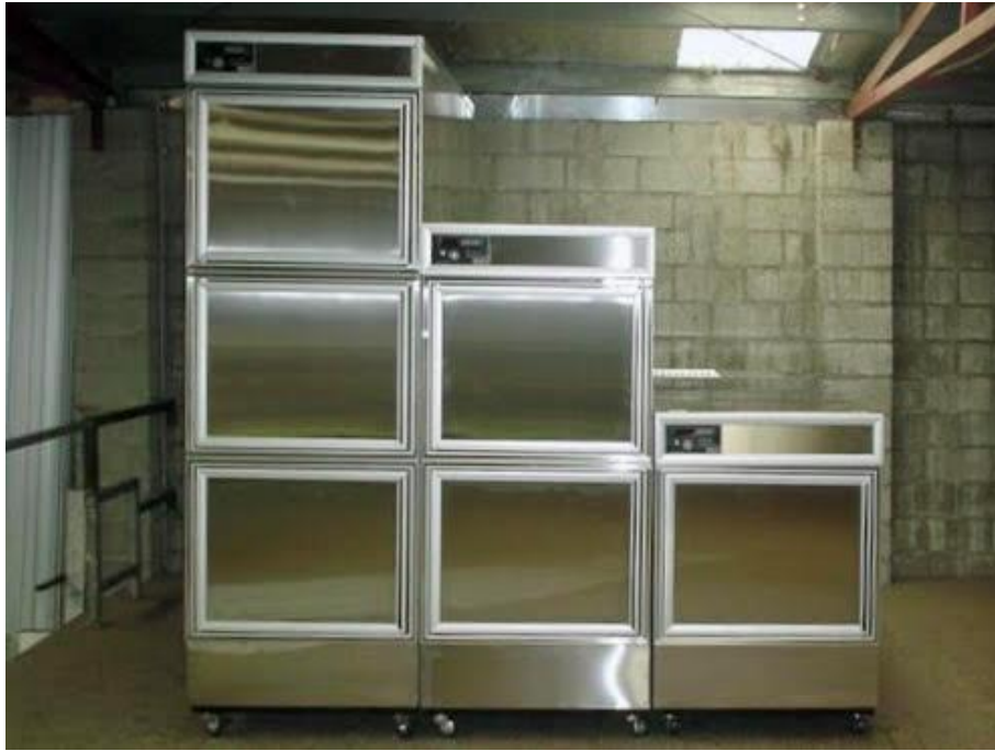
From left to right: 3 berth standard mortuary fridge, 2 berth standard mortuary fridge, 1 berth standard mortuary fridge. Picture taken prior to dispatch, in factory.
